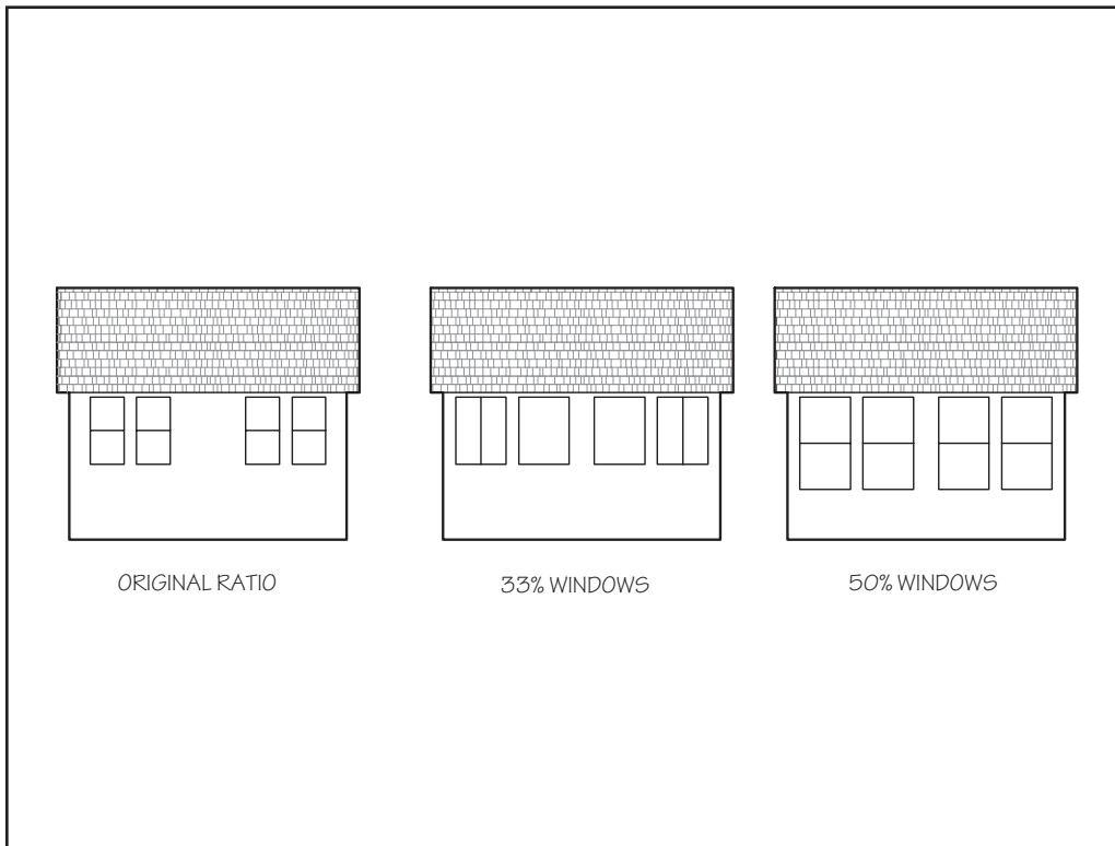
Figure 32—These three drawings show the differences that result from increasing the ratio of openings to solid walls. Noticeably larger ratios produce an incompatible appearance.
